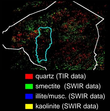
Endmember mapping of the Little Conestoga water shed area illustrates a large amount of smectite. Swelling clays tend to produce water impermeable crusts that increase runnoff, rilling and gully development. The TIR and SWIR data allow for a more complete mineralogical analysis of the the soil including quartz, clays, carbonates and evaporites (Hubbard, 2008). How do changes in land composition affect coastal and inland aquatic ecosystems? [DS 25]
