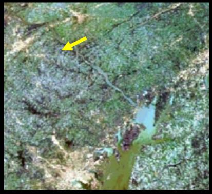
MODIS image (04/09/00) of Chesapeake water shed during heavy rainfall. Yellow arrow illustrates location of increased sediment loading at the Little Conestoga water shed into the Susquehanna River and resulting sediment plume in the upper part of the Chesapeak Bay
